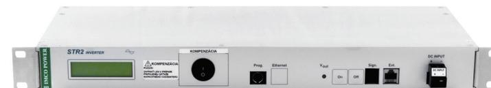
The STR 2 type pure sine wave inverters convert DC 48V (24V) input voltage to 230V ~ 50Hz AC output voltage.
