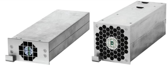
The LS300.Z type rectifier is a plug-in unit for LS1500 chassis. Rectifier modules are built in most advanced technology of the energy conversion with respect to maximum efficiency. The 1U unit provides 48V(12V, 24V) / 350W output, the 2U unit provides 48V(24V) / 700W output power. In LS1500 power supply configuration are rectifiers controlled through LS1500.Z(S) BS management system unit. The fan is temperature controlled.
