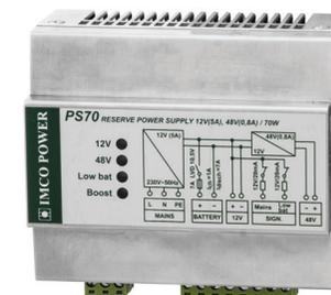
PS70.H backup power supply are designed for reverse supply 12V/5A and 24V/1.5A or 12V/5A and 48V/0.8A. The total output power is 70W. In case of mains failure, the connected 12V battery provides the uninterruptable backup supply of 12V and 24V (48V) load. In case of battery discharge, the power supply will provide its correct disconnection. After the mains powers up, the battery will be automatically recharged to its full capacity.
