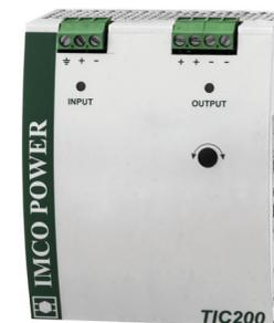
TIC200.H DC/DC converters convert 24V (48V) input voltage to 12V (24V, 48V, 220V) output voltage with galvanic separation. DC/DC converters are equipped with a local LED indication located on the front panel. There is possibility of output voltage trimming (see specification table).
