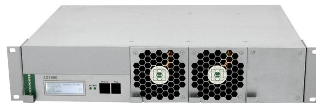
The LS1500 type power sources are designed to back up supply devices and to simultaneously charge the connected battery. In case of mains failure the connected battery continues to supply load without interruption. The power source unit is designed as a plug-in module that can be added or replaced during operation, without a need to turn the system off.
