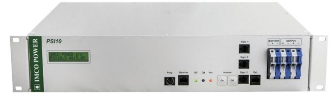
UPS PSI10 type is a backup power supply for 48V (24V) devices and also devices with AC 230V ~ 50Hz input voltage. The advantage of this solution in comparison to conventional UPS is the possibility of connecting a large battery capacity and also devices with DC supply voltage. Especially the UPS can be retrofitted with a 12V or 24V DC/DC converter up to 100W.
