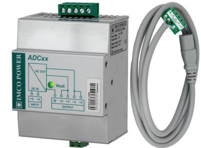
DC/DC converters type ADC01.H convert 48V DC input voltage to 24V DC output voltage. ADC02.H type converters with 24V DC input voltage are designed to supply devices with input voltage 100-230V~50/60Hz up to 100W without needs a DC/AC inverter. For this purpose, a part of the delivery is a special cable for supplying of this device. Output is galvanically isolated from the input, output terminals are doubled. The LED on the front panel indicates the presence of the output voltage.
