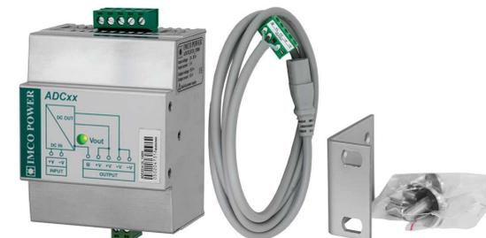
DC/DC converters type ADC01.H convert 48V DC input voltage to 24V DC output voltage. ADC02.H type converters with 24V(48V) DC input voltage are designed for to supply devices with input voltage 100-230V~50/60Hz up to 100W without needs a DC/AC inverter. For this purpose, a part of the delivery is a special cable for supplying of this device. Output is galvanically isolated from the input, output terminals are doubled. The LED on the front panel indicates the presence of the output voltage.
