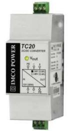
TC20.H DC/DC converters TC20.H type convert 12V(24V) input voltage to 12V (24V, 48V) output with galvanic separation. Converters are equipped with a local LED indication located on the front panel.
