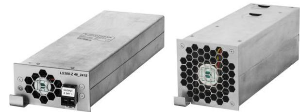
The LS300.Z type rectifier is a plug-in unit for LS1500 chassis. Rectifier units are built in most advanced technology of the energy conversion with respect to maximum efficiency. The 1U unit provides 48V (12V, 24V) / 350W output, the 2U unit provides 48V (24V) / 700W output power. In LS1500 power supply configuration are rectifiers controlled through LS1500.ZS BS management system unit. The fan is temperature controlled.
