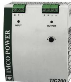
The TIC200.H DC/DC converters convert 24V (48V) input voltage to 12V (24V, 48V, 220V) output voltage with galvanic separation. DC/DC converters are equipped with a local LED indication located on the front panel. There is possibility of output voltage trimming (see specification table).
