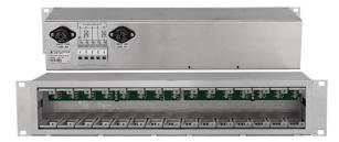
The DL2U PoE / DISTRIBUTION (15x) is a 19 "chassis with a height of 2U (88mm) containing 15 positions for passive PoE.Z 1Gb plug-in unit or DL.Z 24480303 power distribution unit. The individual chassis positions are numbered from 1 to 15. The unoccupied positions can be masked with a blind (set of 10 blinds - not included).
