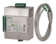
DC/DC converters type ADC02.H with 24V (48V) DC input voltage are designed to supply devices with input voltage 100-230V~50/60Hz up to 100W without needs a DC/AC inverter. For this purpose, a part of the delivery is a special cable for supplying of this device. Output is galvanically isolated from the input. The LED on the front panel indicates the presence of the output voltage.
