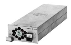
The LS300.Z 48\_2414 DC/DC converter is a hot plug-in unit for LS1500 chassis. The DC/DC converter is built in most advanced ZVS technology with respect to maximum efficiency. The 1U unit provides conversion from 48VDC to 24V/15A with 420W output power. Input filter, output filter, soft start and output trim voltage are standard features for each unit.
