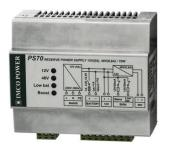
The PS70.H backup power supply is designed for reverse supply 12V/5A and 24V/1.5A or 48V/0.8A. The total output power is 70W. In case of mains failure, the connected 12V battery provides the uninterruptable backup supply on both outputs. When the battery capacity drops to a critical level, the power supply will ensure its correct disconnection. After the mains powers up, the battery will be automatically recharged to its full capacity.
