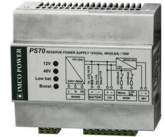
The PS70.H backup power supply is designed for reverse supply 12V/5A and 24V/1.5A or 48V/0.8A. The total output power is 70W. In case of mains failure, the connected 12V battery provides the uninterruptable backup supply on both outputs. When the battery capacity drops to a critical level, the power supply will ensure its correct disconnection. After the mains powers up, the battery will be automatically recharged to its full capacity.
